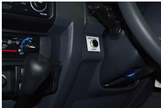
Figure 63: Emergency Start Button
