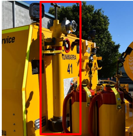
Figure 54: Standpipe – NS on the Rear Deck
