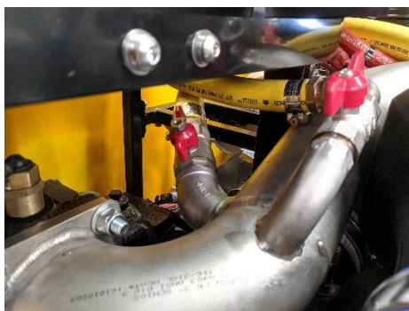
Figure 70: CAFS Mixer Water Isolation Valve
