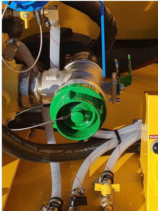
Figure 28: Suction “L” Port Valve (Shown in the “Tank” position).
