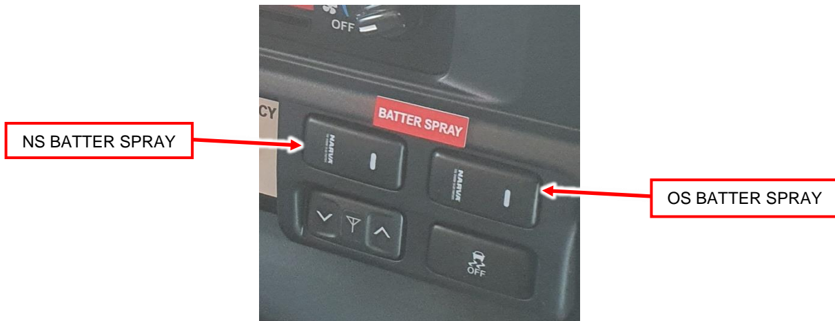
Figure 35: In-cab batter spray switches.
