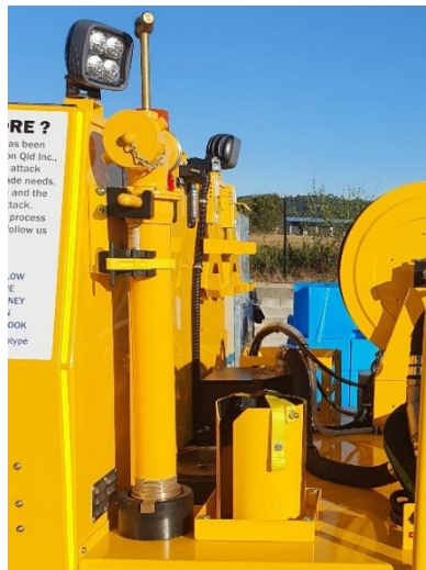
Figure 53: Standpipe and Drip Torch – NS on the rear deck.
